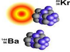
$n + {}^{235}_{92}\text{U} \rightarrow {}^{236}_{92}\text{U} \rightarrow {}^{144}_{56}\text{Ba} + {}^{89}_{36}\text{Kr}$
